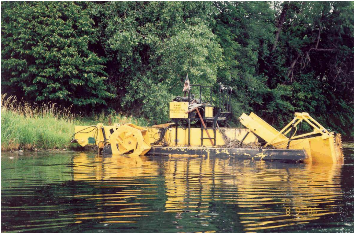
Mechanical harvesting is an option for managing nuisance aquatic plant growth and was used in 2006, 2007, and 2008.
