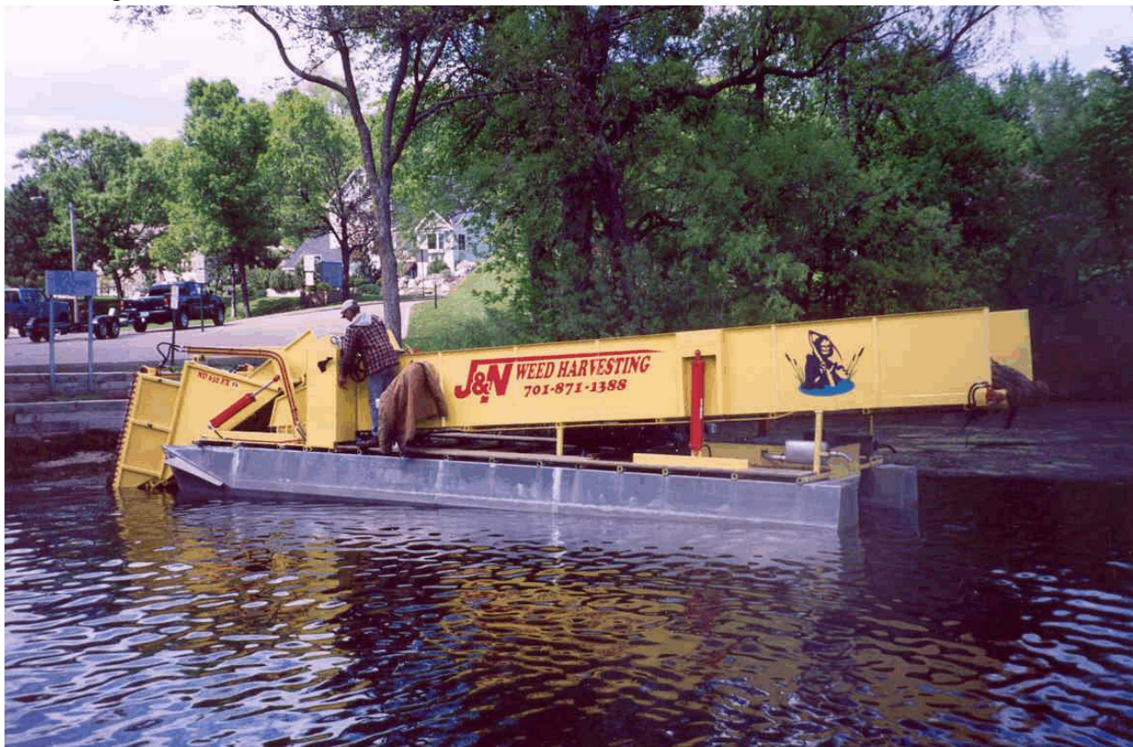
Figure 7. An aquatic plant harvester is an option for curlyleaf control for Schmidt Lake.
