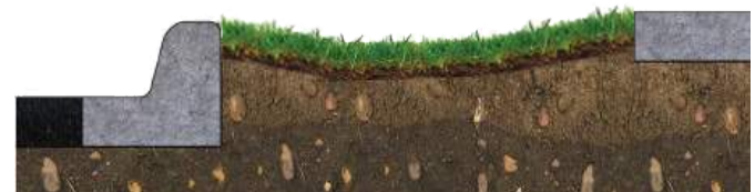
Lowered Turf Boulevard
