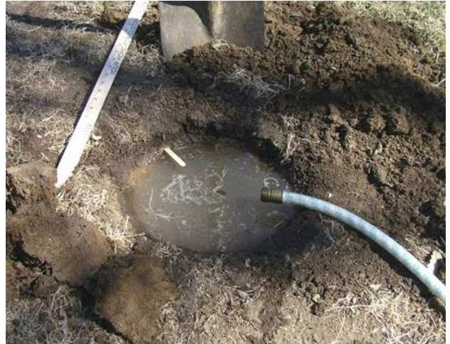
Filling test hole with water
