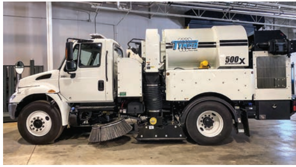
The new sweeper effectively collects pollutants such as fine sediment, salt and debris not captured by standard machines.
