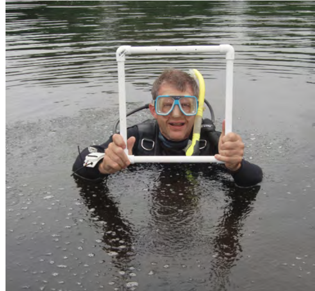
Figure 10. A quadrat is a square frame laid down on the bottom. All plant stems within the 0.1 m 2 square are counted.
